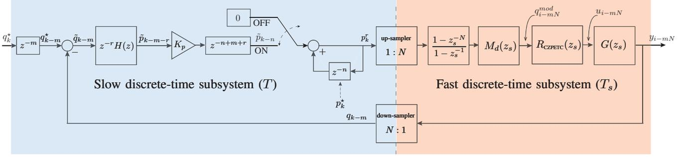
Fig. 10. Practical implementation of the RC scheme based on B-spline trajectory generator and CZPETC for a digitally controlled plant.
